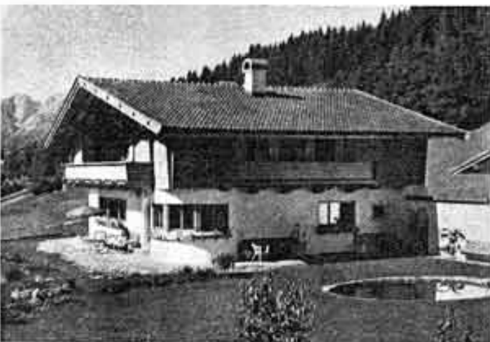
Two views of a comfortable chalet designed for year around enjoyment. The balcony is recessed for greater depth and to give wind protection. The shape of the rounded corner window bay is repeated in arched openings and arched chimney cap.
